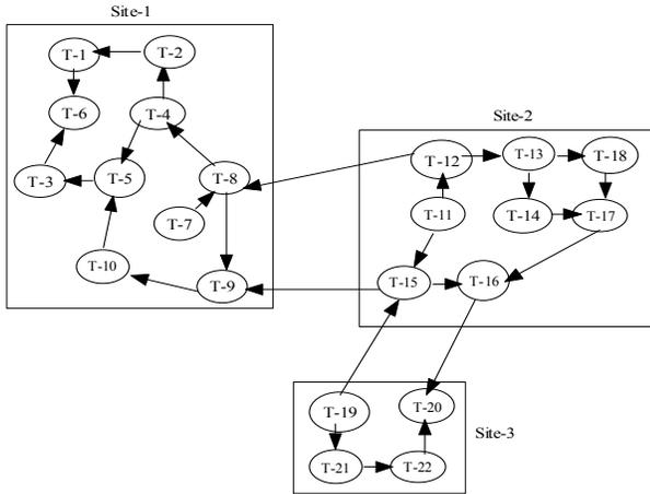
Figure 2. Optimized TWFG free from deadlock within three sites S1, S2 and S3.
