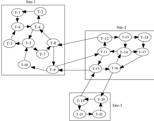
Figure 1. Complex TWFG consist local and global deadlock within three sites S1, S2 and S3.
