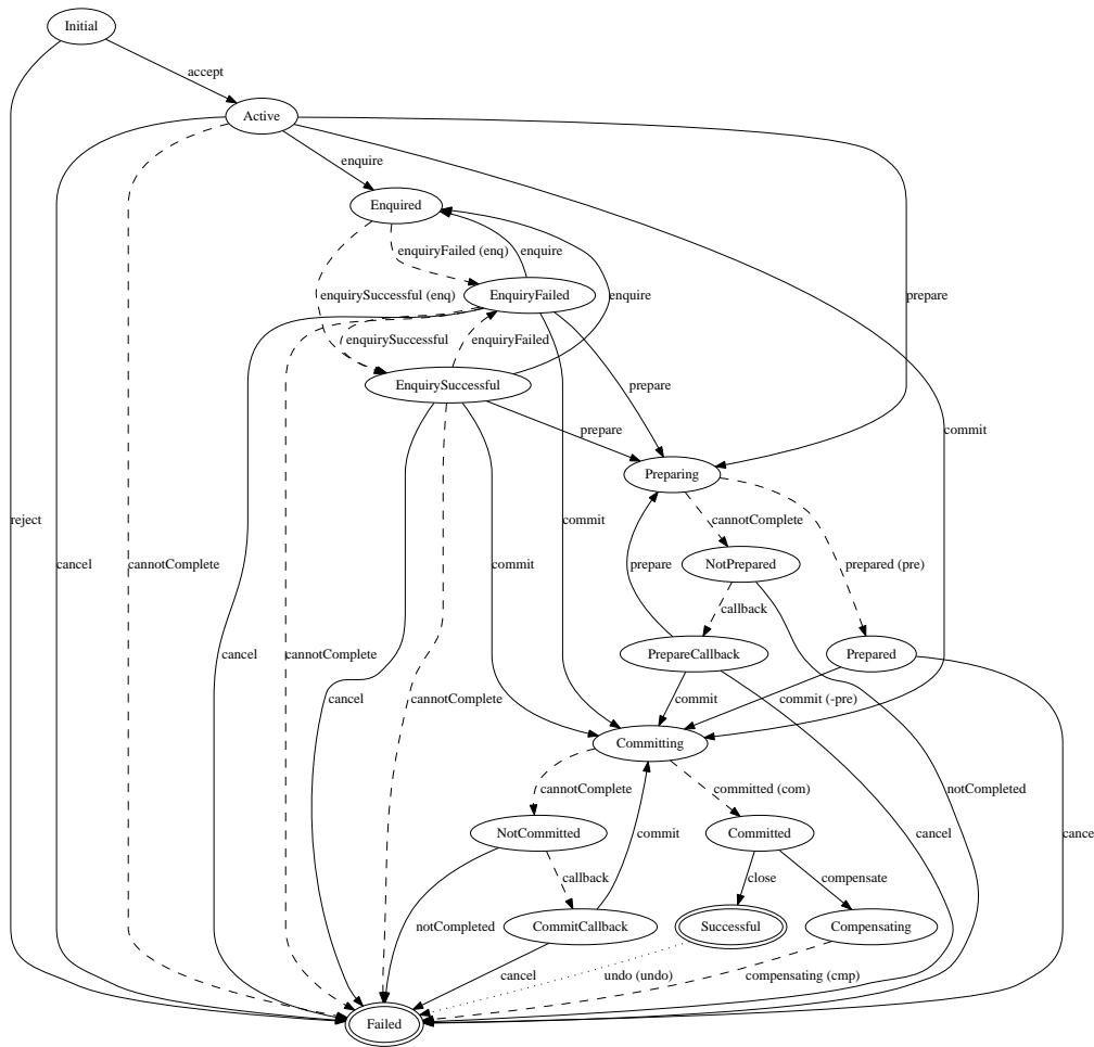
Figure 1: State transition diagram for a client’s processing of an activity. Solid lines represent messages sent by the client. Dashed lines represent messages sent by the service provider. Dotted lines indicate client-side only transitions. Values in parentheses represent the associated cost to the client.
